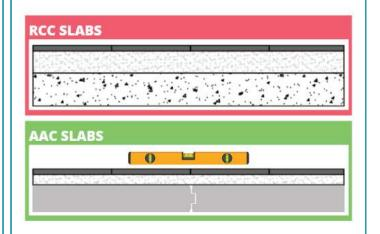
Being uniform floor area, reduces the quantity for bedding material for tiles. Thereby reducing the dead weight on slab & reduces cost of bedding material.
